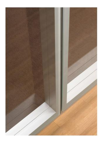
The supporting substructure consists of floor- and ceiling-mounted profiles that hold supporting steel mullions. The glazed elements on both sides are single-pane or laminated safety glass panes that are glued with a two-component adhesive onto an aluminium frame that runs around the rear and inserted into the mullion construction. The wall thickness is 100 mm, or 125 mm where requirements for sound insulation and/or statics are higher.
